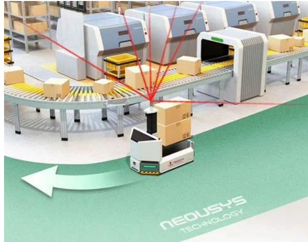
Vision guided systems utilize computer vision to interpret the surroundings of the AGV
